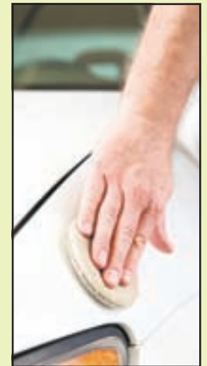
Washing off harmful substances promptly can reduce the chances of damage to a paint job.
