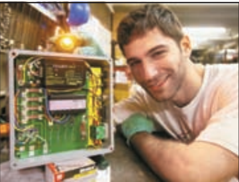
Denos "DJ" Vourderis shows the LED system behind the Wonder Wheel's solar-powered lights.
