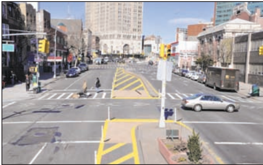
LEFT TURN BANS: The city-proposed plan would eliminate eight left turns along Fourth Avenue. The city would widen narrow pedestrian islands from two feet to up to 19 feet at intersections where turns are made illegal by the use of paint and bollards.
