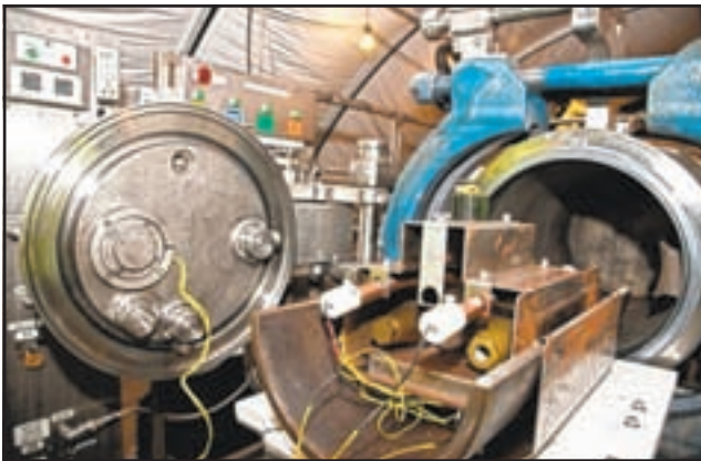
CONTROLLED DEMOLITION: The explosive destruction system is a safe and effective means of destroying chemical munitions. The blast and vapor are contained inside the chamber. U.S. Army
